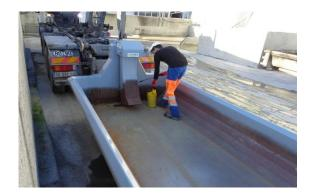
The bottom of the bucket is made of 6 mm anti-abrasion sheet in one piece with reinforcing support cross members. This guarantees its flatness over time. In addition, the very flared and rounded shape of the product allows a low tilt of emptying to avoid jerks and overturning of the truck.
