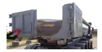
The sealing of the double doors makes it possible to contain the laitance of the concrete as well as the anhydrite screed. The low deformation of these double doors makes it possible to guarantee their tightness over time, which limits the risk of slipping around the skip.
