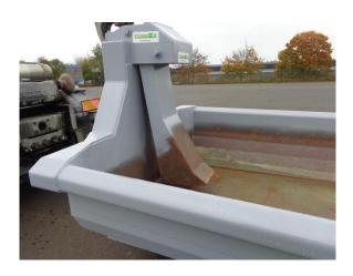
The upper edges of the CEMBOX are inclined towards the inside of the skip to collect any pieces of hardened concrete which can become detached by vibrations during transport.
