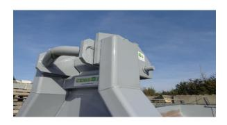
Now it moves away from the front face as soon as the CEMBOX tipper is empty, which allows the mold release oil to be sprayed without muscular effort.
